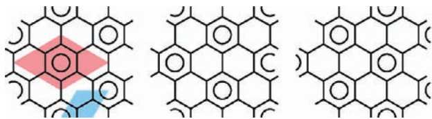
Figure 4. The three equivalent Clar formulas of graphene. At the left, the primitive unit cell of graphene is shown in blue and the unit cell of the (\sqrt{3} \times \sqrt{3})R30^\circ superstructure is shown in red. Note that only a subsection of the infinite graphene lattice is shown.
